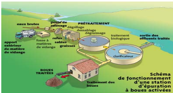
Figure – Activated sludge station diagram.
